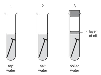
In which test-tubes do the nails rust?
